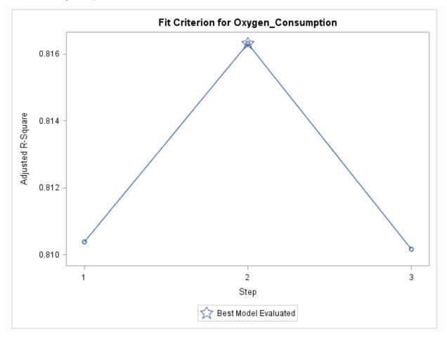
The Adjusted R-Square for the model at step 2 (before **Weight** was removed) was greatest of the three tested. Note the scale of the Y-axis for Adjusted R-Square. The differences in value among the three values is minimal. A [0-1] scale for the access would have shown how small the differences truly are.
