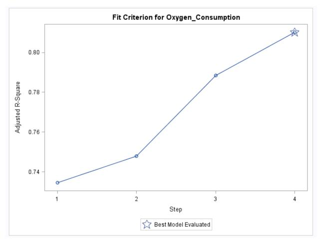
The default entry criterion is  $p \le .50$  for the forward selection method and  $p \le .15$  for the stepwise selection method. After **RunTime** was entered into the model, **Age** was entered at step 2 with a *p*-value of 0.1222. If the criterion were set to something less than 0.10, the final model would have been quite different. It would have included only one variable, **RunTime**. This underscores the precariousness of relying on one stepwise method for defining a "best" model.
