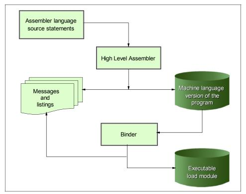
Figure 2-1 Assembler source to executable module
