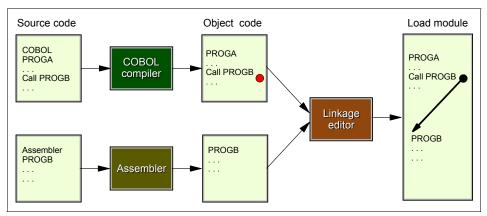
Figure 3-3 Resolving references during load module creation
