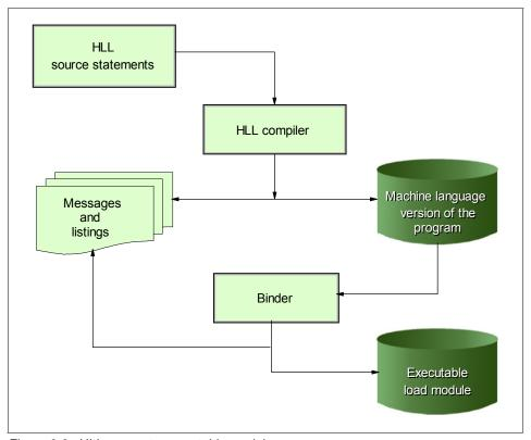
Figure 2-2 HLL source to executable module
