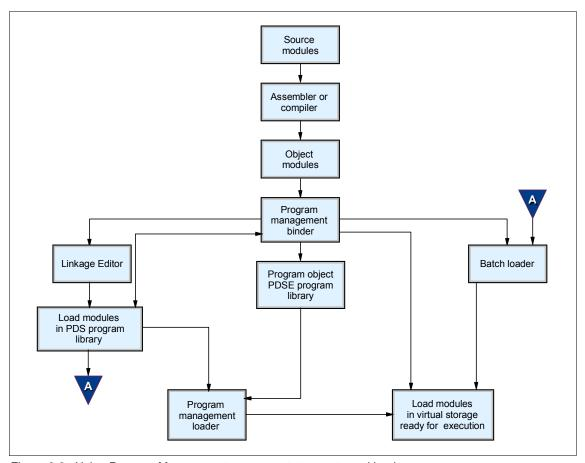
Figure 3-2 Using Program Management components to create and load programs
