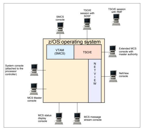
Figure 1-5 Sample console configuration for a z/OS system
