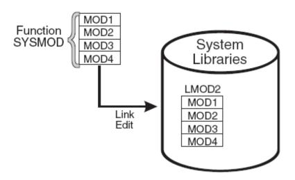
The above figure shows the installation of a function SYSMOD links-edits object modules MOD1, MOD2, MOD3 and MOD4 to create load module LMOD2. The executable code created in load module LMOD2 is installed in the system libraries through the installation of the function SYSMOD.
