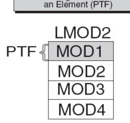
In the above diagram we see a previously installed load module, LMOD2. If we want to replace the element MOD1, we should install a PTF SYSMOD that contains the module MOD1. That PTF SYSMOD replaces the element in error with the corrected element. As part of the installation of the PTF SYSMOD, SMP/E relinks LMOD2 to include the new and corrected version of MOD1.
