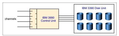
Figure 3-7 Initial IBM 3390 disk implementation
