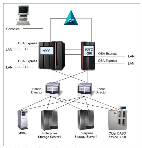
Figure 3-14 Moderately large mainframe configuration
