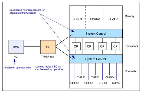
Figure 3-6 System control and partitioning
