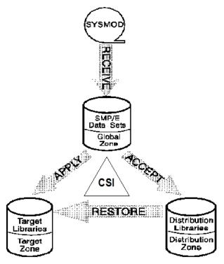
Figure 2-6 Flow of SMP SYSMOD Processing
