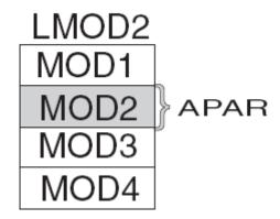
The processing of the APAR SYSMOD provides a modification for the object module MOD2. During the installation of the APAR SYSMOD, MOD2 is updated (and corrected) in LMOD2.
