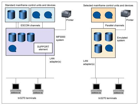
Figure 3-12 Very small mainframe configurations
